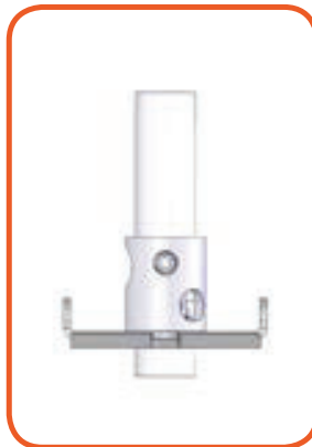
Air hole blocked - Back in NG position
