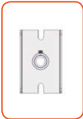
Air inlet of Venturi in NG position
