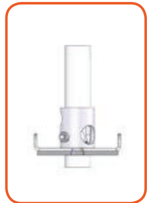
Air inlet hole - Back in LPG position
