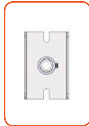
Air inlet of Venturi in LPG position
