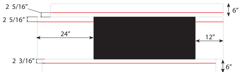
Layout Lines for the Scaffold 95
