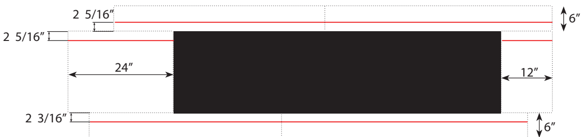
Layout Lines for the Scaffold 185
