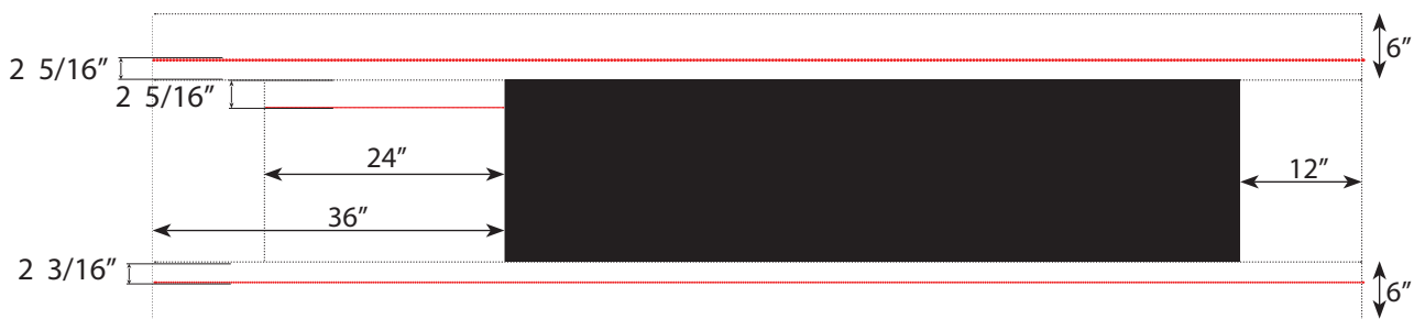
Layout Lines for the Fulcrum 72 (not to scale) (red lines for z-clips)
