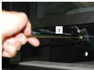
Figure 34g. Removing and installing the glass doors. (both sides typical)
