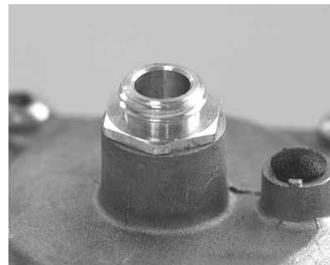
Figure A6 - Close-up of Regulator Cap Set to LP
